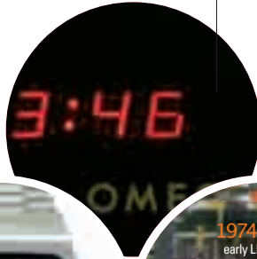
1974 Close up of Omega LED watch revealing each individual LED 'dot'
